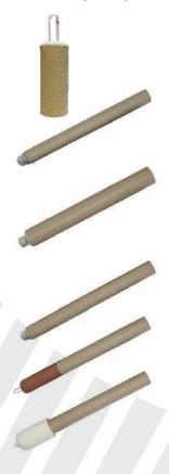
**BMD Tips** These can be used 6 to 8 times to measure temperature of molten metal in slag free condition. This tip is having ceramic tube.
