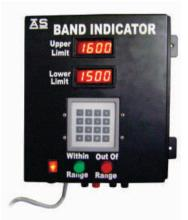
It is a microcontroller based, wall mountable unit which is used for giving audio and visual indication for Within Range Temperature Reading (Green Lamp) and Out of Range Temperature Reading (Red Lamp + Hooter). It has facility to enter Upper Limit Reading and Lower Limit Reading of Temperature.
