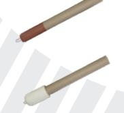
**Safe Tip** The anti-splash tip is manufactured with a special coating that prevents molten metal from spurting and splashing. Due to extra protection this thermocouple is usable 8 to 10 times, reducing the cost of each reading.
