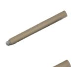
**MINI Tips** These are expendable cardboard sleeve tips useful to measure temperature of molten metal with slag. It has Male Receptacle. Expendable Mini Tip is available in different lengths having ID 18 mm & OD 32 mm.
