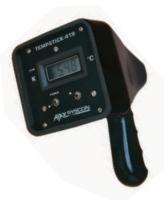
Model 419K is an accurate temperature measuring instrument. This pyrometer is specially designed to measure temperature of non ferrous molten metal upto  $1000^{\circ}$ C
